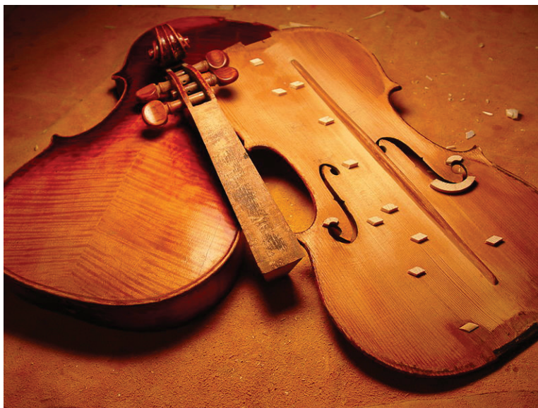
Figure 74: Inside a violin – you can see the bass bar on the inside face of this violin body
